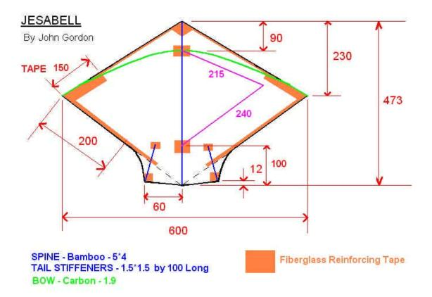
I think the bow diameter and the spine dimensions are in millimeters as are the dimensions of the kite. Bruce
